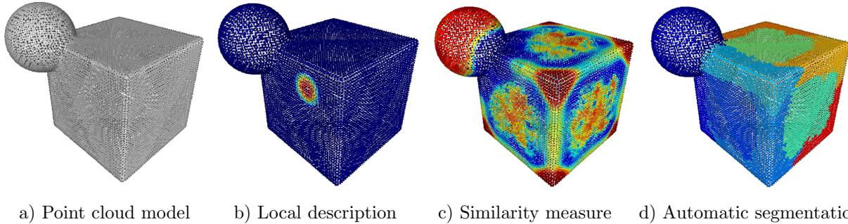
Figure 1: These images, generated by our Matlab code, show each of the stages of our point cloud model analysis procedure, from model to SPCL to an HKS vector to one of many possible segmentations.
