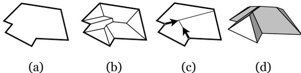
Figure 1: (a) A polygon, (b) its straight skeleton, (c) its induced motorcycle graph, and (d) its straight skeleton roof.
