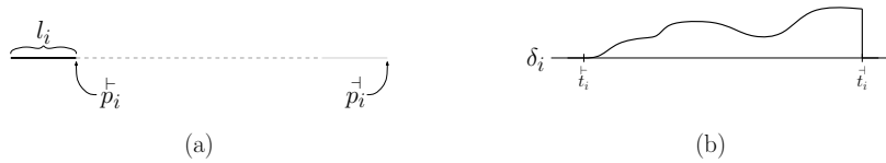
Figure 1: (a) The physical specification of a vehicle v_i . (b) A possible speed profile, \delta_i , for a vehicle v_i .
